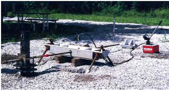
LATERAL LOAD TEST APPARATUS FIGURE B-6
