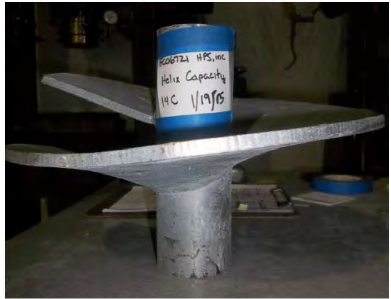
FIG. C-2 - RS2875 14" DIA. HELIX - TEST RESULTS
